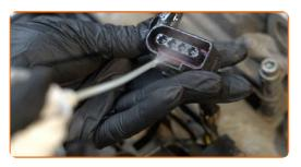
Plug in the connectors of the ignition coils.
