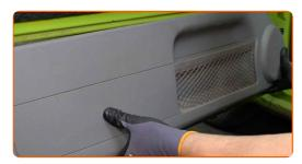
Screw in the fasteners of the lower door card. Use a Phillips screwdriver.
