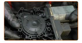
Install and screw in the motor fasteners on the new window regulator mechanism. Use a Phillips screwdriver.
