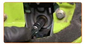
Disconnect the glass from the window regulator mechanism.
