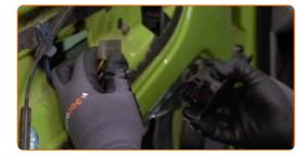
Unscrew the fasteners of the window regulator assembly. Use a drive socket #10. Use a ratchet wrench.
