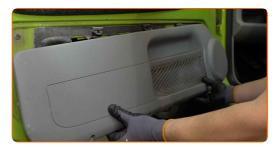
Remove the power window switch module. Use a plastic trim tool.
