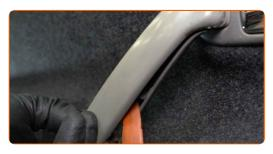
Unscrew the door handle fastener. Use a Phillips screwdriver.
