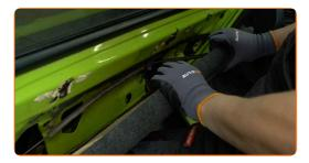
9 Remove the handle-to-lock cable.
