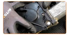
Treat the power window motor connector. Use dielectric grease.
