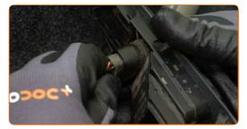
Install the power window switch module.
