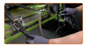
Unscrew the power window motor fasteners. Use a Phillips screwdriver.
