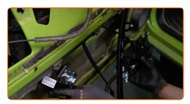
Screw in the fasteners of the window regulator mechanism. Use a drive socket #10. Use a ratchet wrench.
