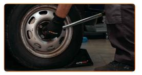
Tighten the wheel bolts using a criss-cross pattern. Use wheel impact socket #17. Use a torque wrench. Tighten it to 110 Nm torque.
