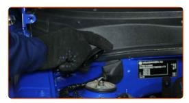
Unscrew the top fastening of the shock strut mount. Use a combination spanner #21. Use HEX No.H7. Use a ratchet wrench.
