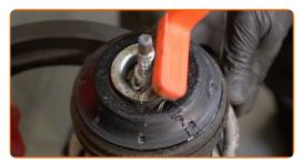
Remove the strut piston rod nut. Use a drive socket #21. Use HEX No.H7. Use a ratchet wrench.
