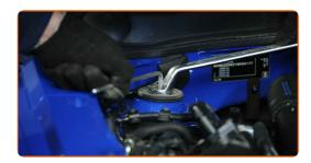
Install the protective shock absorber mounting cap.
