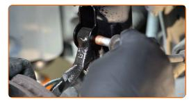
Tighten the lower fasteners connecting the shock strut to the steering knuckle. Use a combination spanner #18. Use a drive socket #18. Use a torque wrench. Tighten it to 40 Nm torque.+90°
