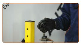
Tighten the shock strut piston rod nut. Use a drive socket #21. Use HEX No.H7. Use a torque wrench. Tighten it to 60 Nm torque.
