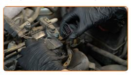
Clean dirt, dust and debris from inside the spark plug wells.
