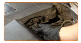
Remove the engine cover assembled with the air filter housing.
