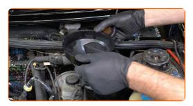
Pour coolant in the coolant reservoir.
