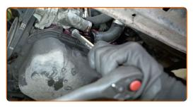
Remove the thermostat housing.
