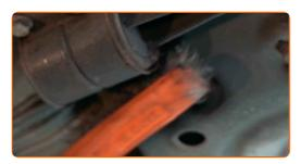
Unscrew the fasteners that connect the gearbox mount to the subframe. Use a drive socket #13. Use a ratchet wrench.
