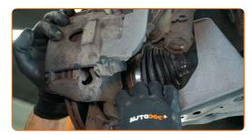
Attach the ball joint to the control arm. Use a pin punch.
