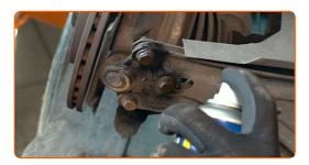
Unscrew the fastener connecting the ball joint to the suspension control arm. Use a drive socket #13. Use a ratchet wrench.
