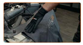
Unscrew the fasteners of the car battery terminals. Use a drive socket #10. Use a ratchet wrench.
