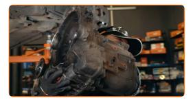
Remove the release bearing. Use a crowbar.
