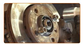
Screw in the nut of the CV axle. Use a drive socket #30. Use a ratchet wrench.
