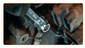
Unscrew the ground wire fastener. Use a combination spanner #13.
