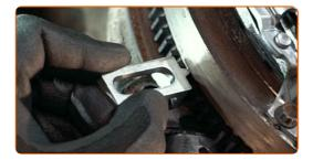
Tighten the pressure plate fasteners. Use 12-point socket No.9. Use a torque wrench. Tighten it to 27 Nm torque.
