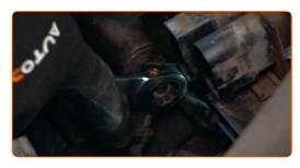
Treat the engine wiring harness connectors. Use dielectric grease.
