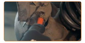
Unscrew the brake caliper fastening. Use HEX No.H6. Use a ratchet wrench.
