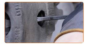
10 Remove the brake caliper.
