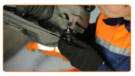
Tighten the ball joint fastener. Use a drive socket #13. Use a torque wrench. Tighten it to 20 Nm torque.+90°
