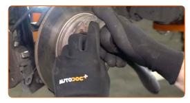
15 Remove the brake disc.
