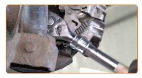
Release the parking brake cable. Use water pump pliers. Use a crowbar.
