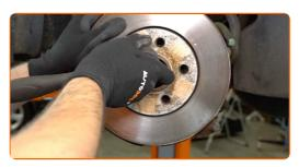
16 Remove the brake disc.
