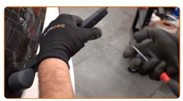
Press the clip. Use a flat screwdriver. Remove the blade from the wiper arm.
