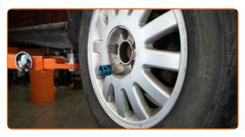
Lower the car and working in a cross order, tighten the wheel bolts. Use a torque wrench. Tighten it to 120 Nm torque.
