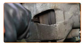
Remove the brake caliper.
