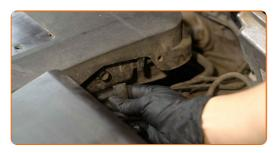
Remove the engine cover assembled with the air filter housing.
