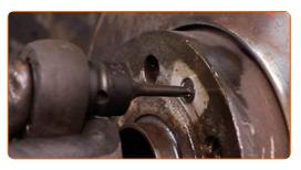
17 Remove the brake disc.
