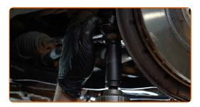
Tighten the tie rod end locknut. Use a combination spanner #24 (2 pieces). Use a torque wrench. Tighten it to 50 nm torque.
