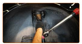
Tighten the lower fastener of the shock absorber. Use a drive socket #21. Use a torque wrench. Tighten it to 180 Nm torque.
