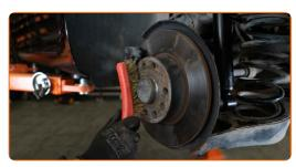
Treat the contacting surface. Use copper grease.
