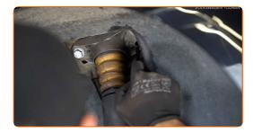
Tighten the shock absorber mount fasteners. Important! Be sure to use new fasteners. Use a drive socket #16. Use a torque wrench. Tighten it to 50 Nm torque.+45°
