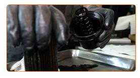
14 Remove the oil filter cover O-ring.
