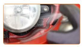
5 Unscrew the fog light fasteners. Use Torx T20.
