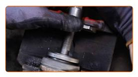
18 Install the brake caliper guide pins.
