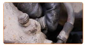
Install the brake caliper retaining spring.
