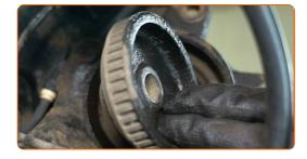
Remove the wheel hub. Use the hub slide hammer puller.
