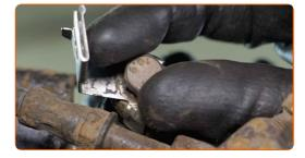
Tighten the brake caliper fasteners. Use a combination spanner #15. Use a drive socket #13. Use a torque wrench. Tighten it to 35 nm torque.
