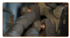
Tighten the brake caliper bracket fasteners. Use a drive socket #18. Use a torque wrench. Tighten it to 110 nm torque.
