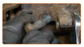
Remove the brake caliper. Use a crowbar.
