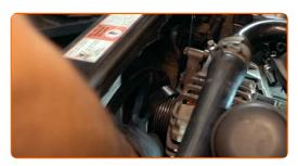
Replacement: engine thermostat – SEAT Alhambra (7V8, 7V9). Tip from AUTODOC:
