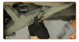
Screw the fasteners of the stabilizer bush brackets. Use a drive socket #13. Use a torque wrench. Tighten it to 35 nm torque.
