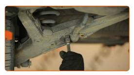
Remove the stabilizer bush brackets. Use a flat screwdriver.
