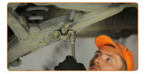
Treat the fasteners of the stabilizer bush brackets. Use copper grease.
