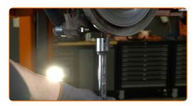
Unscrew the lower fastener of the shock absorber. Use a combination spanner #21. Use a drive socket #21. Use a ratchet wrench.
