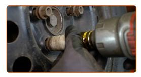
Lower the car and working in a cross order, tighten the wheel bolts. Use wheel impact socket #19. Use a torque wrench. Tighten it to 170 Nm torque.
