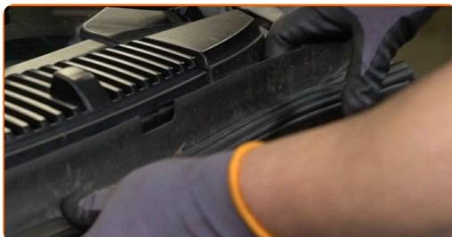
**5** Unscrew the plastic panel fasteners. Use a drive socket #10. Use a ratchet wrench.
