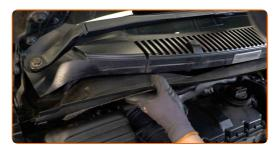
Screw on the plastic panel fasteners. Use a drive socket #10. Use a ratchet wrench.
