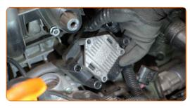
Install the new ignition coil to the spark plug well.
