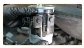
Put the old filter cartridge in the container.
