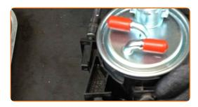
Clean the fuel filter pipe. Use all-purpose cleaning spray.
