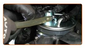
Connect the pipe to the fuel filter.
