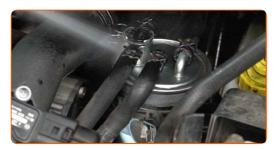
Loosen the fastening clamps of the fuel filter pipes. Use clic-R collar pliers.
