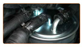
Attach the fuel pipe clamp. Use clic-R collar pliers.
