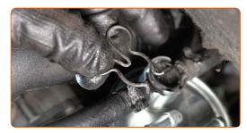
Disconnect the pipe from the fuel filter.
