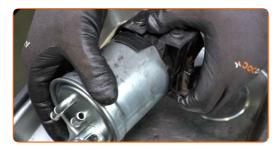
13 Install the bracket onto the new filter.
