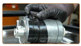
Unscrew the bracket fastener. Use a drive socket #8. Use a ratchet wrench.
