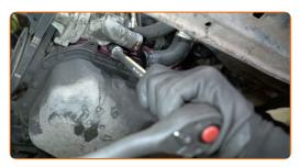
Remove the thermostat housing.
