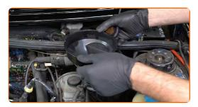
Pour coolant in the coolant reservoir.
