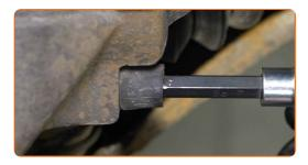
11 Remove the brake caliper.
