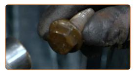
19 Remove the caliper bracket.
