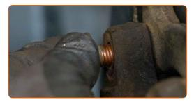
Tighten the brake caliper bracket fasteners. Use a drive socket #18. Use a torque wrench. Tighten it to 110 nm torque.
