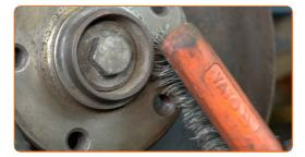
Treat the contacting surface. Use ceramic grease.
