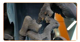
Clean the brake disc fastener. Use a wire brush. Use WD-40 spray.
