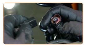
Clean the brake caliper retaining spring. Use a wire brush. Use a brake cleaner.
