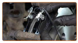
37 Install the brake caliper and fix it.
