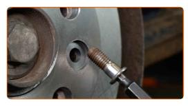
Tighten the brake disc fastening. Use HEX No.H6. Use a torque wrench. Tighten it to 10 Nm torque.
