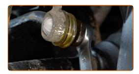
Unscrew the fastener connecting the stabilizer link to the shock strut. Use a combination spanner #16. Use a drive socket #19. Use a ratchet wrench.
