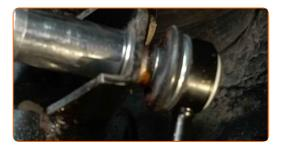
Tighten the fastener connecting the stabilizer link to the stabilizer bar. Use a drive socket #17. Use a torque wrench. Tighten it to 100 Nm torque.
