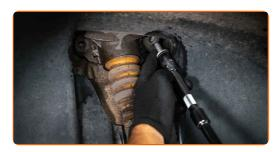
Unscrew the lower fastener of the shock absorber. Use a combination spanner #21.
