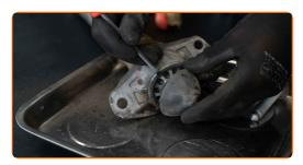
Remove the shock absorber piston rod fastening. Use a combination spanner #16. Use an adjustable wrench.
