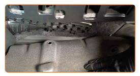
A Remove the cabin filter housing cover.
