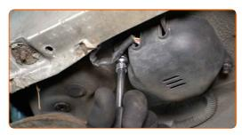
Remove the oxygen sensor housing cover.
