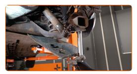
Unscrew the lower fastener of the shock absorber. Use a combination spanner #18. Use a drive socket #18. Use a tap wrench. Use a ratchet wrench.
