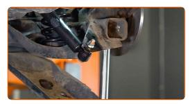
Tighten the lower fastener of the shock absorber. Use a combination spanner #18. Use a drive socket #18. Use a torque wrench. Tighten it to 105 Nm torque.
