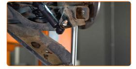
Tighten the lower fastener of the shock absorber. Use a combination spanner #18. Use a drive socket #18. Use a torque wrench. Tighten it to 105 Nm torque.
