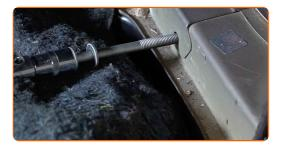
Remove the shock absorber. Use a crowbar.
