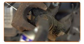
Press in the brake caliper piston. Use brake caliper wind back tool.
