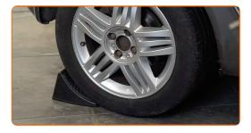
Loosen the wheel mounting bolts. Use wheel impact socket #19.
