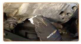
Screw in the new drainage plug and tighten it. Use square oil drain plug socket No.8 Use a torque wrench. Tighten it to 20 nm torque.
