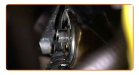
Lubricate the rubber seal of the new filter with a little amount of fresh oil.
