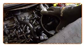
Pour oil into the engine through the filler. Required amount of oil: 4.8 L.
