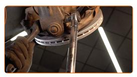
Tighten the lower fasteners connecting the shock strut to the steering knuckle. Use a drive socket #18. Use a torque wrench. Tighten it to 105 Nm torque.
