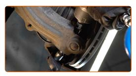
Remove the fastening bolt.
