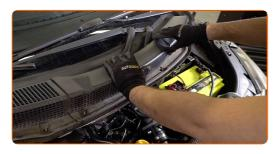
Screw in the fastener of the wiper cowl grille located on the left side. Use a drive socket #10.
