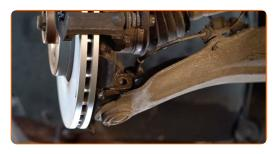
Disconnect the ball joint from the steering knuckle. Use a crowbar.
