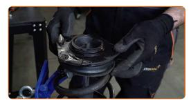
Tighten the shock strut piston rod nut. Use a combination spanner #19. Use HEX No.H6. Use a torque wrench. Tighten it to 60 Nm torque.
