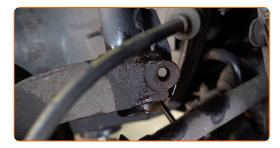
Treat the shock strut fasteners. Use WD-40 spray.
