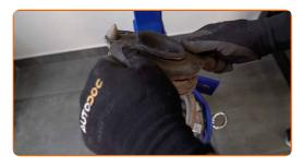
Release the coil spring.
