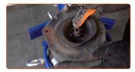
Remove the strut piston rod nut. Use a combination spanner #19. Use HEX No.H6.
