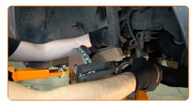
Unscrew the lower fastener connecting the shock strut to the steering knuckle. Use a drive socket #18. Use a tap wrench.
