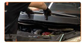
6 Unscrew the fastener of the wiper cowl grille located on the right side. Use Torx T20.
