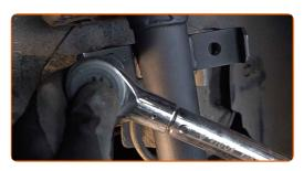
Treat the shock strut fasteners. Use copper grease.
