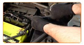
Raise a little the top protective cover. Remove the air filter housing.
