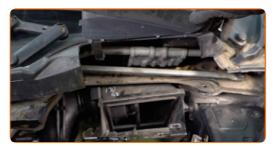
Reinstall the air filter housing.
