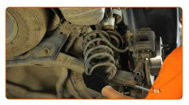
Remove the rubber spring spacer.
