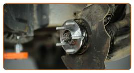
Tighten the wheel hub nut. Use a drive socket #32. Use a torque wrench. Tighten it to 195 Nm torque.
