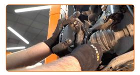
Tighten the brake caliper bracket. Use a combination spanner #17. Use a drive socket #17. Use a torque wrench. Tighten it to 85 Nm torque.
