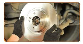
Tighten the brake disc fasteners. Use a Phillips screwdriver. Use a torque wrench. Tighten it to 6 Nm torque.
