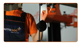
Tighten the fastener connecting the stabilizer link to the stabilizer bar. Use a combination spanner #17. Use a drive socket #17. Use a torque wrench. Tighten it to 65 Nm torque.
