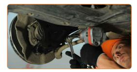
Tighten the fastener connecting the stabilizer link to the shock strut. Use a combination spanner #17. Use a drive socket #17. Use a torque wrench. Tighten it to 65 Nm torque.
