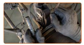
Clean the ABS sensor fastener. Use WD-40 spray.
