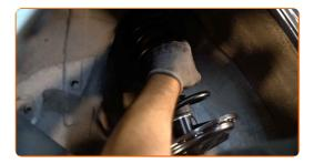
Screw the top fastening of the shock strut mount. Use a drive socket #14. Do not tighten it.
