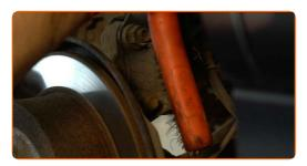
Clean the fastener of the bracket that connects the brake hose to the shock strut. Use a wire brush. Use WD-40 spray.
