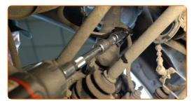
Loosen the fastener that connects the suspension strut to the rear knuckle. Use a combination spanner #19. Use a drive socket #19. Use a ratchet wrench.
