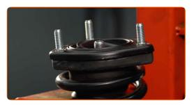
Tighten the shock strut piston rod nut. Use a chain wrench. Use a drive socket #19. Use a torque wrench. Tighten it to 60 Nm torque.
