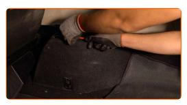
Loosen the upper fastener of the shock strut mount. Use a drive socket #14. Use a ratchet wrench.
