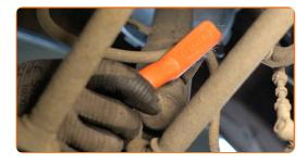
Unscrew the brake hose fastening bracket from the shock strut. Use a drive socket #12. Use a ratchet wrench.
