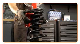
Remove the assembled shock strut.
