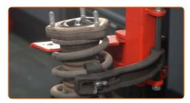
Remove the strut piston rod nut. Use a chain wrench. Use a drive socket #19. Use a ratchet wrench.
