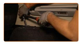
Install the suspesion strut mount cap.
