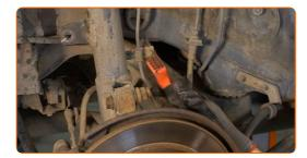
Unscrew the ABS sensor fastener. Use a drive socket #10. Use a ratchet wrench.
