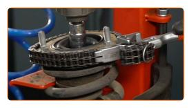
Release the coil spring.
