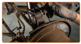
Tighten the fastener that connects the suspension strut to the rear knuckle. Use a drive socket #19. Use a torque wrench. Tighten it to 180 Nm torque.
