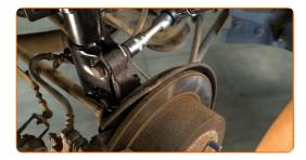
Screw in the ABS sensor fastener. Use a drive socket #10. Use a ratchet wrench.
