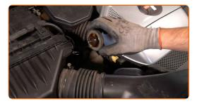
Tighten the oil filler cap.
