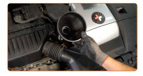
Pour oil into the engine through the filler. Required amount of oil: 4.9 l.
