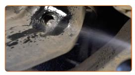
Unscrew the drain plug. Use a combination spanner #14. Use a drive socket #14. Use a ratchet wrench.
