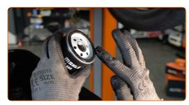
Screw the new filter into its place. Use the 76-14F socket. Use a torque wrench. Tighten it to 23 Nm torque.
