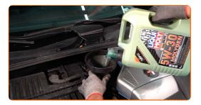
Replacement: engine oil and filter – Lexus RX XU30. Tip:
