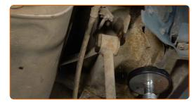
Clean the mounting seats and the thread of the suspension arm. Use a wire brush. Use WD-40 spray.
