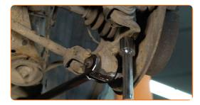
Screw in the fastener that connects the control arm to the rear knuckle. Use a combination spanner #18. Use a drive socket #E18. Use a tap wrench.
