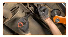
Tighten the fastener connecting the suspension arm to the rear knuckle. Use a combination spanner #18. Use a drive socket #E18. Use a torque wrench. Tighten it to 80 nm torque.
